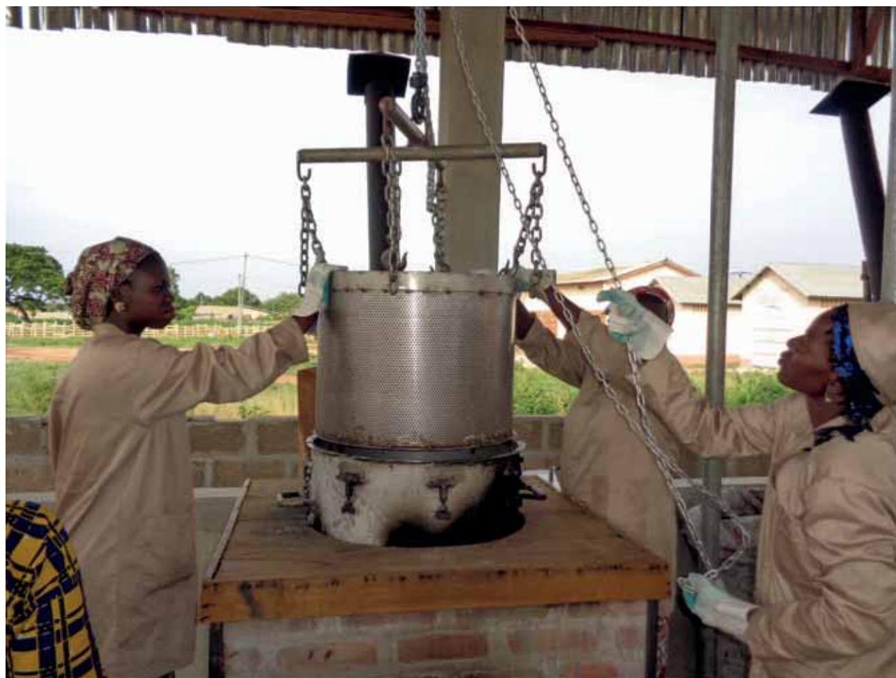
The pulley–hoist and efficient stove help make the GEM setup safer for operators
